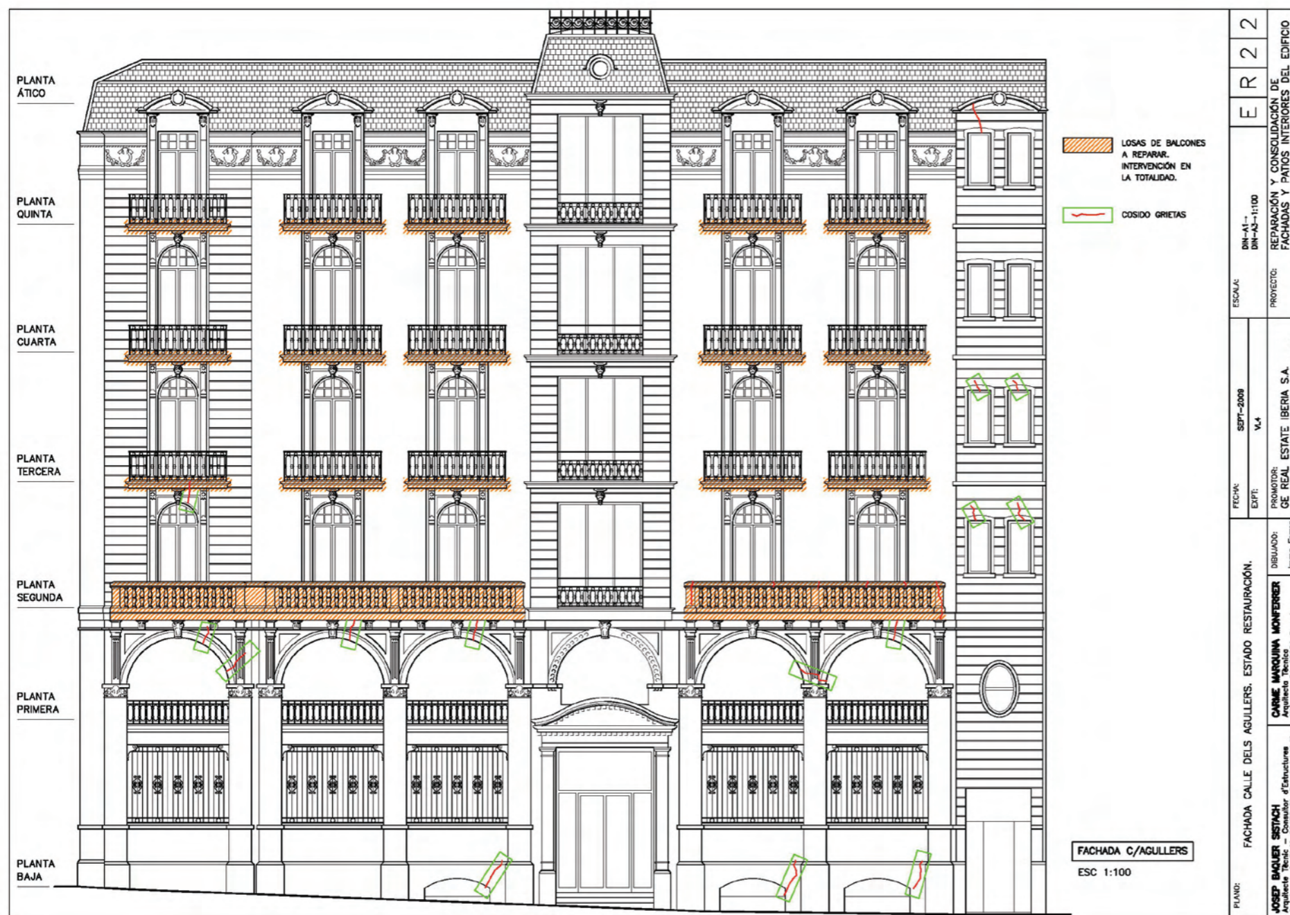
Fig.8: Agullers Street's façade: map of lesions/damages.
