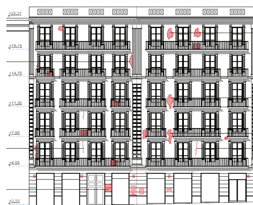
Fig.4: Detail of the damages and issues on the façades, to be repaired.
