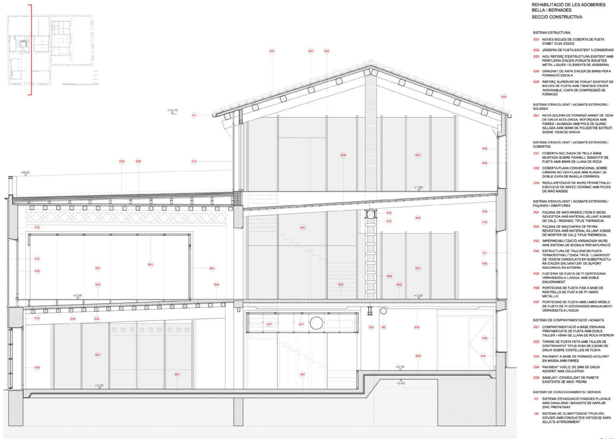
Fig.27: Constructive section. © Taller 9s Arquitectes
