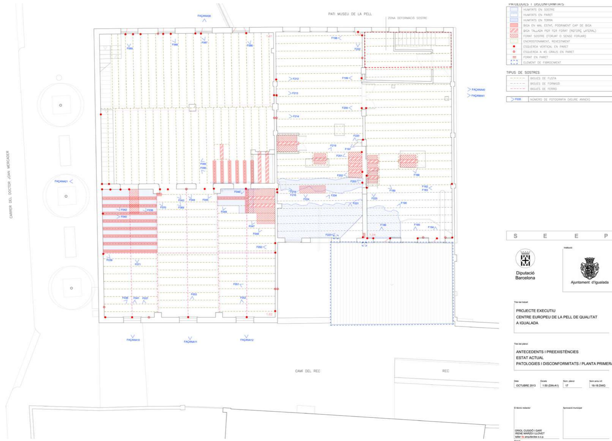
Fig.20: Pathologies and disconformities. First floor ceiling.. © Taller 9s Arquitectes
