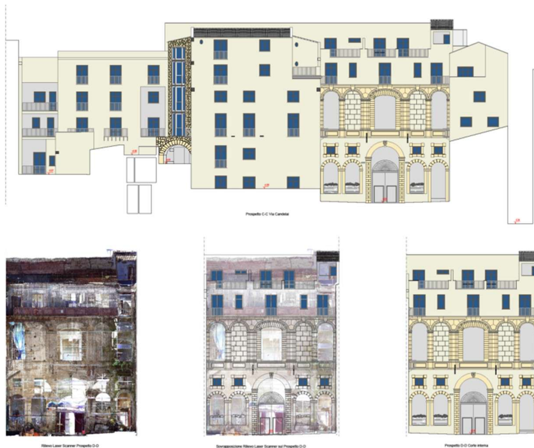
Fig.18: Palace's façade along Calderai Street: from the laser scanner to the project's hypothesis. © Arch. Francesco Miceli
