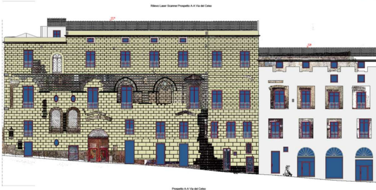
Fig.4: Palace façade along Celso Street: from the laser scanner survey to the façade reconfiguration's design hypothesis. © Francesco Miceli
