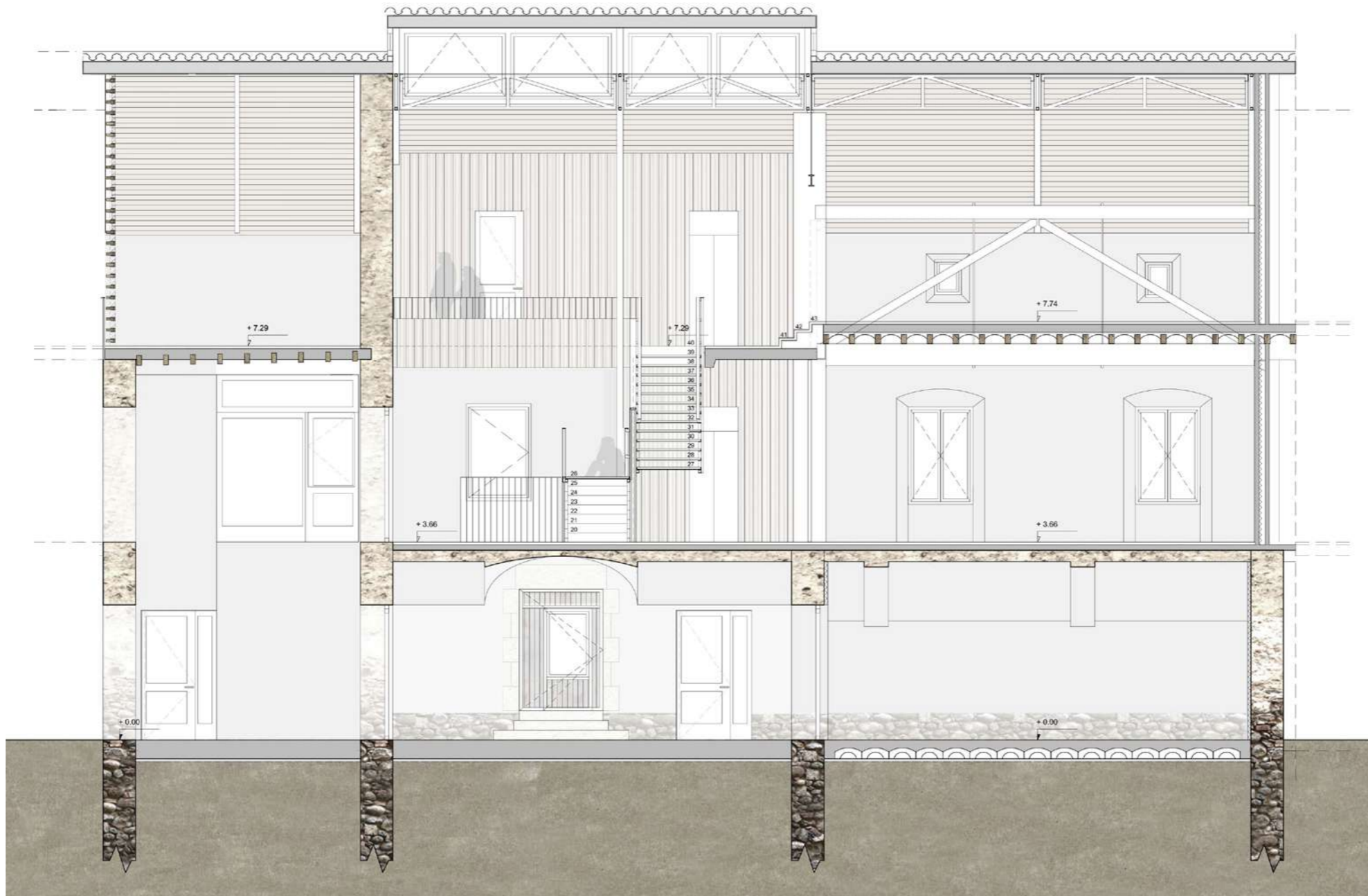
Fig.23: Longitudinal section with the concatenation of double height spaces: main access and new void under the skylight.
