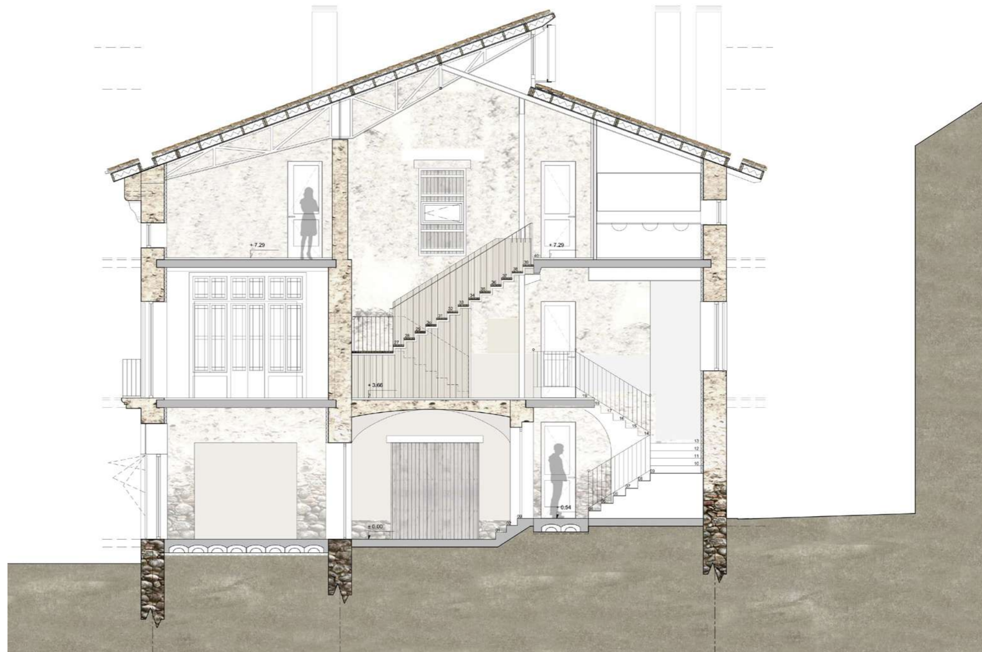
Fig.24: Cross-section in the relation between the old, restored staircase and the new staircase in the central space under the skylight.
