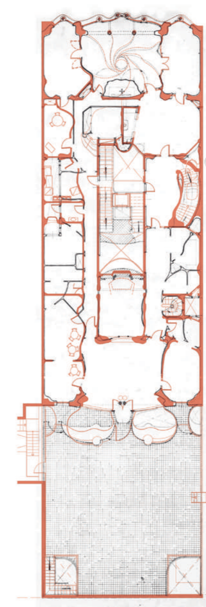
Fig.3 Main floor layout plan: superposition in red from the 2014 survey, in black, drafted by the Friends of Gaudí. Joan Olona, Mireia Bosch
