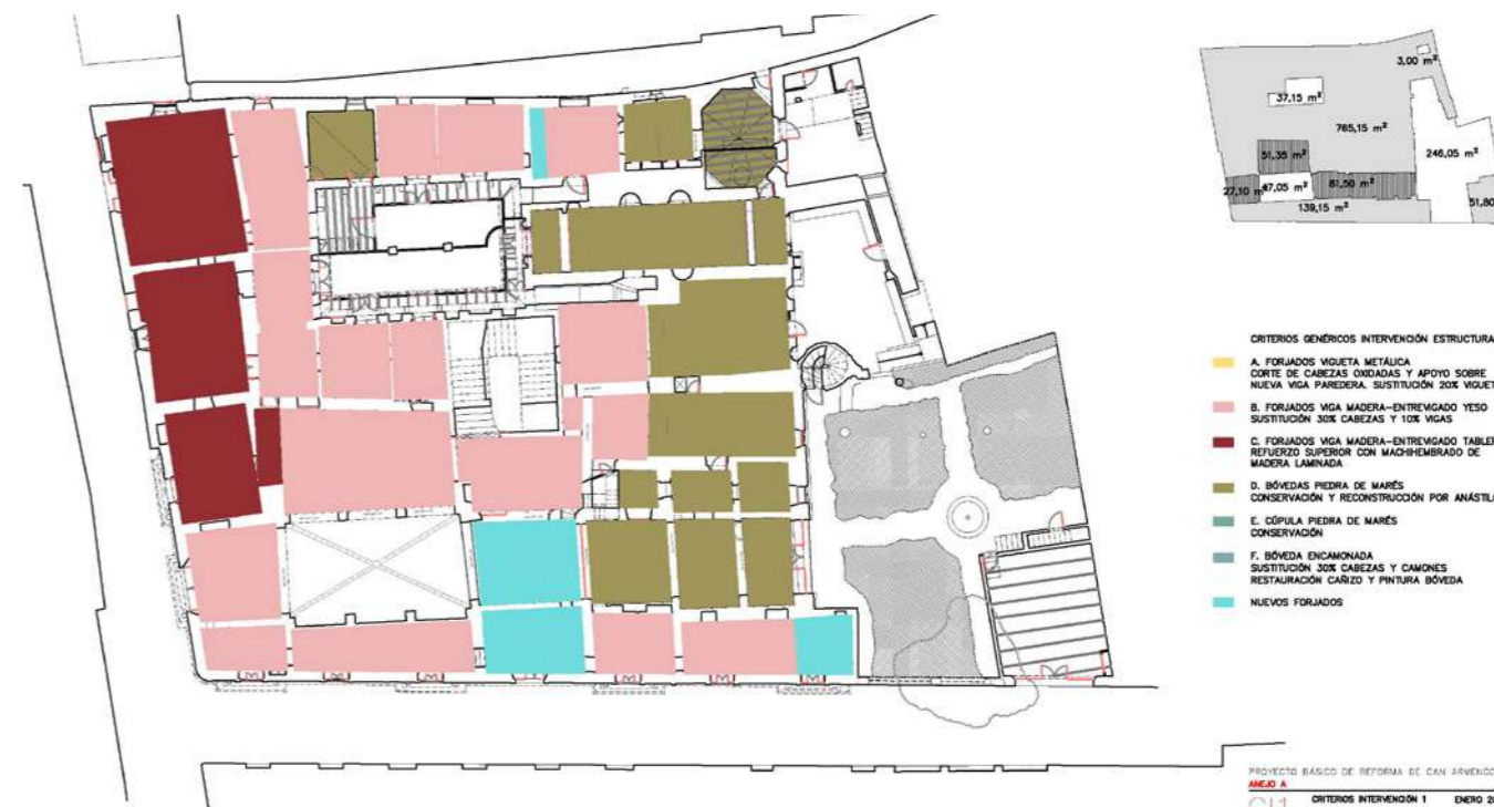
Fig.24: Floor slabs intervention.
