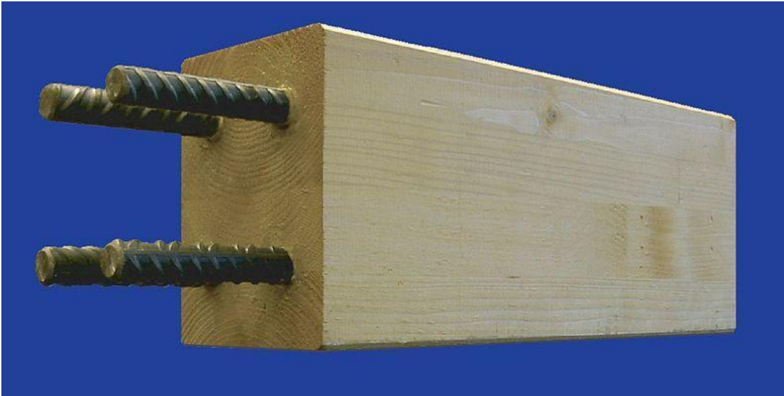
Fig.1: The reinforced beam is obtained by reinforcing the classic glulam wood with the insertion of one or more steel bars in special longitudinal millings made in some lamellas and joined to them. © https://buildingcue.it/cose-il-legno-armato/10917/
