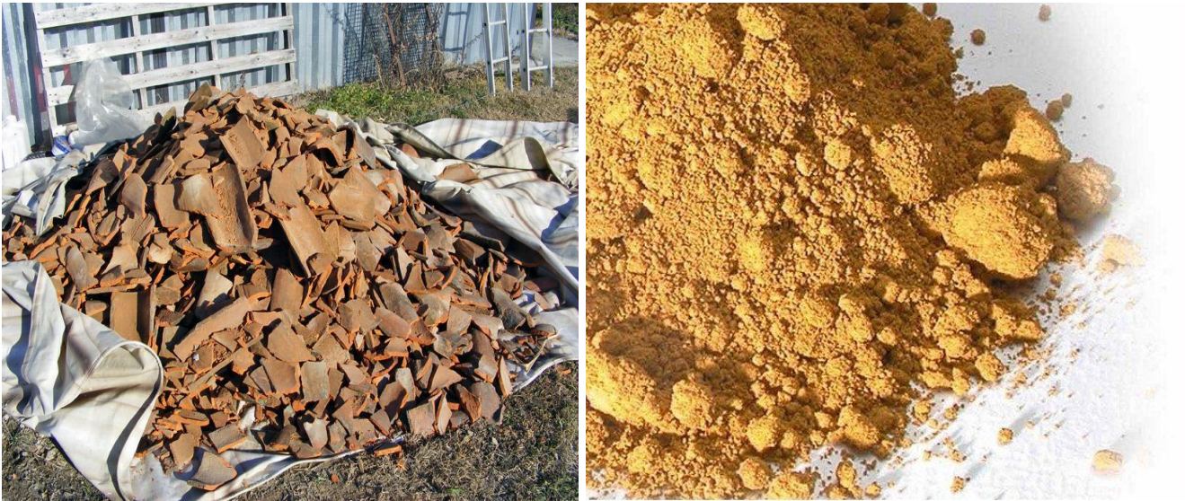
Fig.15-16: Fragments of brick (fig.15). Cocciopesto powder (fig.16). © https://dianti.it/boutiquedellacalce/index.php/calce-uso/il-cocciopesto ; https://www.edilportale.com/prodotti/sandtex/crushed-and-dishydrated-coccio-powder/cocciopesto-cc_362201.html
