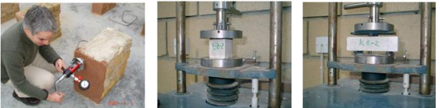
Fig.4: Examination of its mechanical properties of hydraulic plasters. ©Maria Philokyprou
