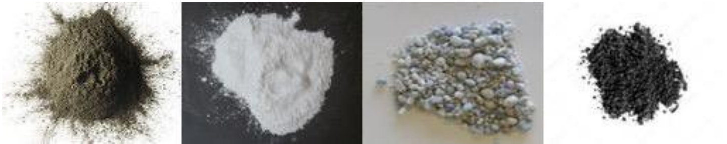
Fig.1: Possible wastes from the paper-pulp industry: (from left) Biomass Fly Ash, Calcareous Sludge, Grits, and Dregs.
