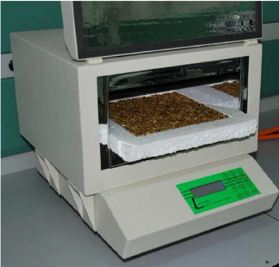
Fig.5: Thermal insulation test. ©Simona Colajanni
