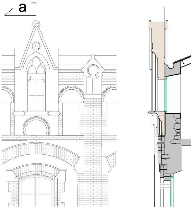
Fig.5: Elevation and section of the decorative element to be consolidated, where its weaker points can be easily appreciated. ©Josep Baquer
