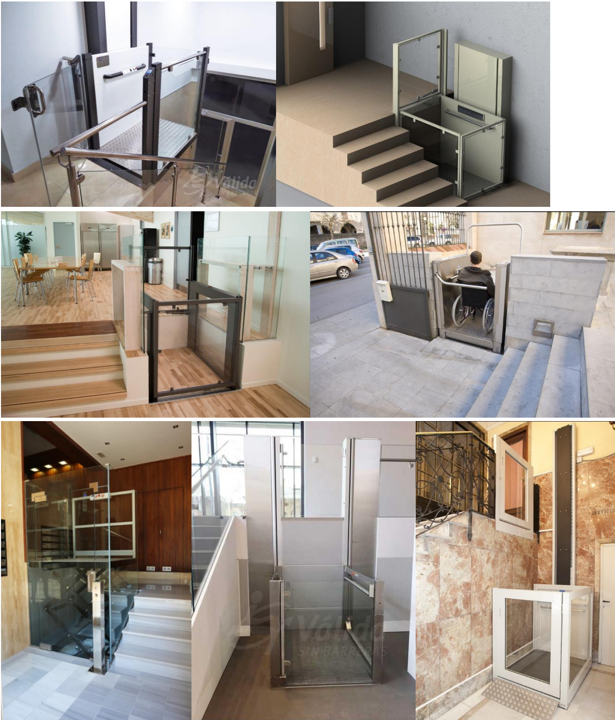
Fig.15-21: Examples of short-travel elevators ideal for wheelchairs to overcome low difference in height. It also doubles as a small cargo elevator, in some cases. It's available in different arrangement of installations, it can be attached to a single point in the wall, in an independent support structure, on exteriors or interiors, with a chain or belt lifting system or with a crane-like lifting system. ©Válidasinbarreras
